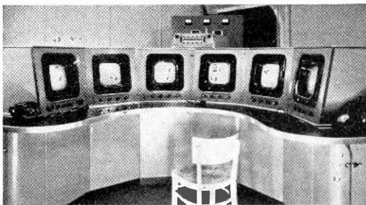
Display console with centralized operating controls.
